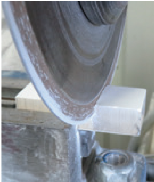
Green machining (cutting) of compacted GRANALOX® .
