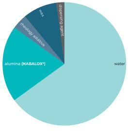
Exemplary formulation of a typical car paint polishing paste
