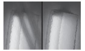
Car paint before (left) and after (right) scratch removal
