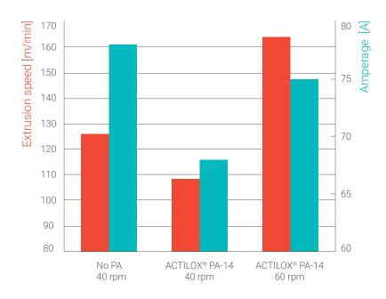
Extrusion speed and amperage during extrusion of a LSFOH compound; Left without, middle and right with ACTILOX® PA-14.
