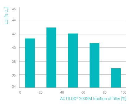
LOI as a function of the mineral filler composition (total filling level 61.3 wt.-%); LOI development by a successive exchange of **APYRAL® 60CD** with **ACTILOX® 200SM** in an EVA compound.
