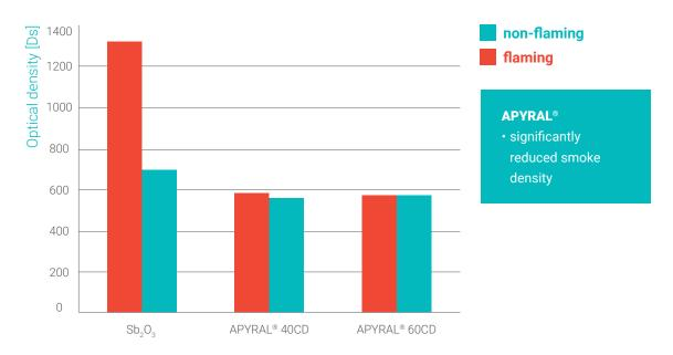
Maximum smoke density according to ASTM E662 of plasticized PVC using different flame retardants.
