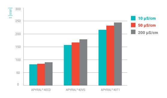
Stability measurement via dehydrochlorination (DHC) test of PVC compounds filled with 80 phr of various  ${\bf APYRAL}^{\circledast}$  grades.
