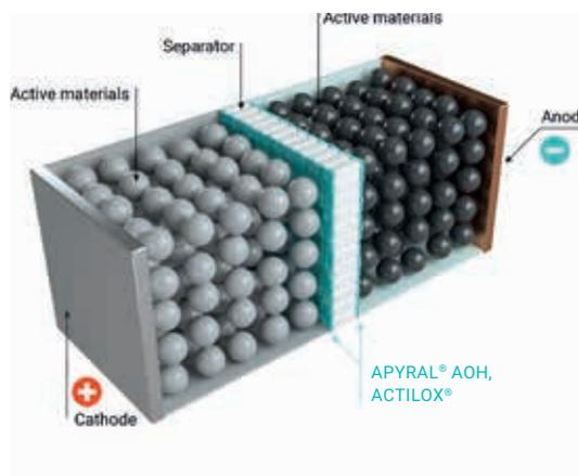
**Figure 3:** Three-dimensional structure illustration of a Lithium-ion battery cell, highlighting the coating of the separator (green).
