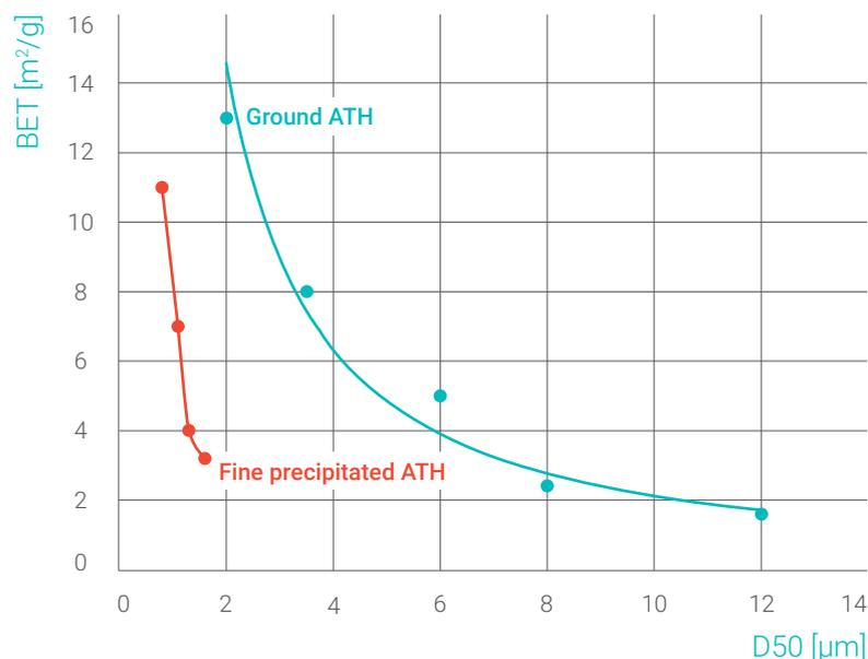
Figure 1: Correlation between D50 and BET of fine precipitated and ground ATH.
