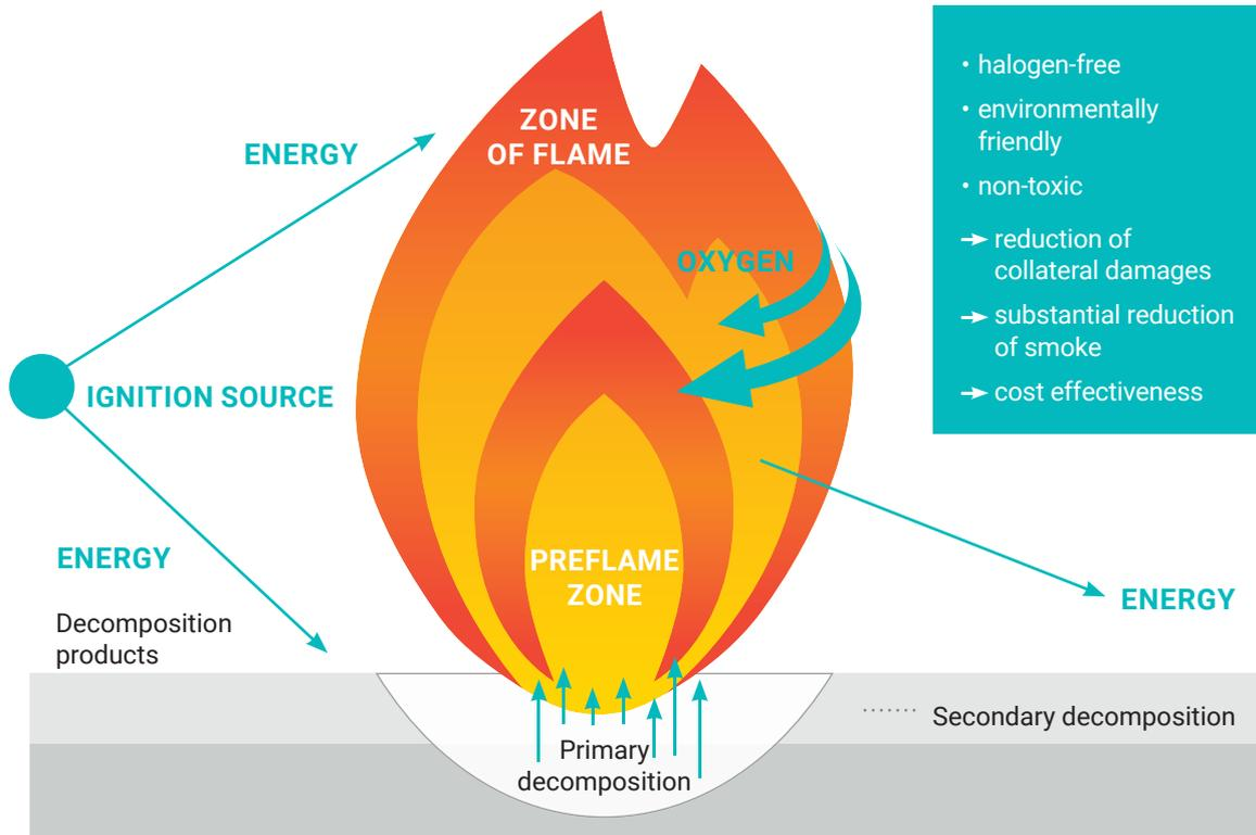
Scheme of the processes involved during burning of an **APYRAL**<sup>®</sup> filled polymer.
