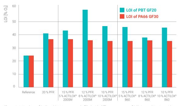
**Figure 3:** LOI values of PBT and PA66-compounds filled with different amounts of PFR in combination with boehmite (**ACTILOX® 200SM** or **ACTILOX® B60**).
