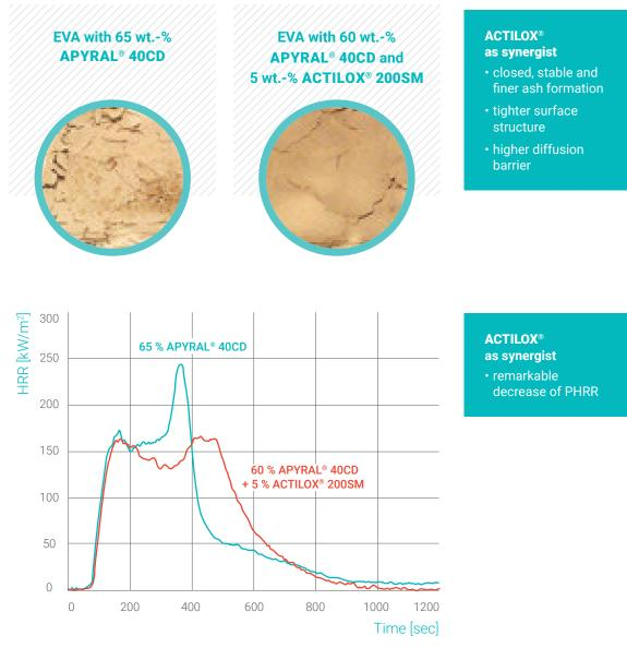
Heat Release Rate (HRR) and Total Heat Released (THR) of EVA compounds filled with 65 wt.-% of metal hydrates.
