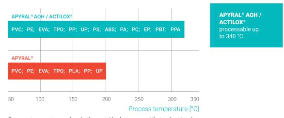
Process temperatures wherein the metal hydrates can withstand and typical polymers in which these fillers can be used.
