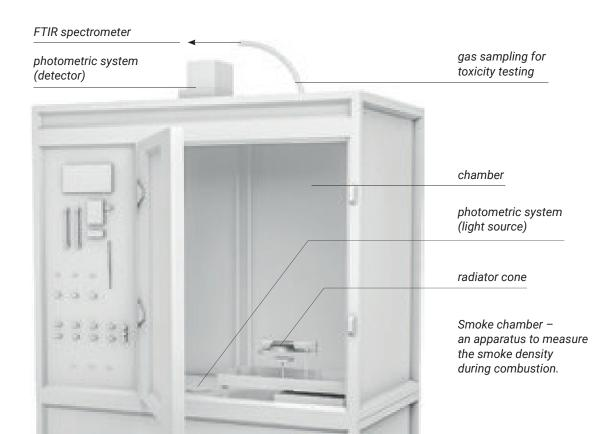
This records the release of smoke over time on the basis of the optical density. The optical density is derived from the smoke released from the specimen into a sealed box which weakens the transmission of a laser beam traversing the box. The more smoke develops in the course of the test, the lower the transmission and thus higher is the optical density.
