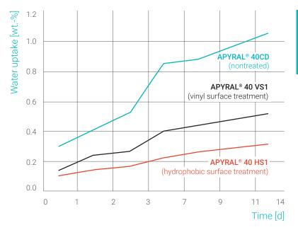
Reduced compound water uptake by hydrophobic surface coating of **APYRAL**®
