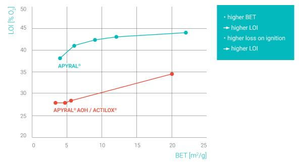
LOI-values of EVA compounds (61.3 wt.-% metal hydrate) depending on the specific surface area of the metal hydrate.
