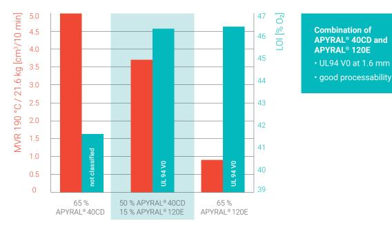
High fire resistance combined with good processability. LOI-values, the UL94 V classification for specimen of 1.6 mm thickness and the melt volume rate (MVR) of EVA compounds filled with **APYRAL**<sup>®</sup> are displayed.
