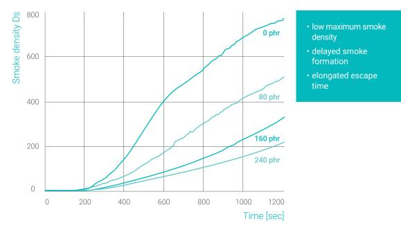
Smoke Density versus filler loading **APYRAL® 20X** in UP-resin according to ISO 5659-2, no pilot flame.
