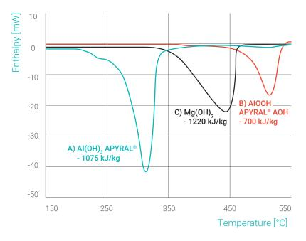
Differential scanning calorimeter data (DSC) of the mineral flame retardants **APYRAL®**, **APYRAL® AOH** and magnesium hydroxide **Mg(OH)**<sub>2</sub>.
