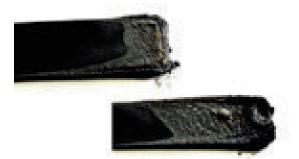
Specimen of glass fibre reinforced PA 6 (GF: 22.5 wt.-%) filled with DEPAL (13.5 wt.-%) and **ACTILOX® 200SM** (5 wt.-%) passes UL94 V0 at 0.8 mm.
