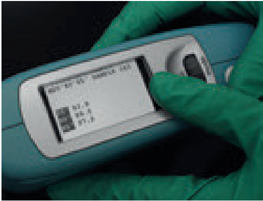
Gloss meter (GU: Gloss Units; Measuring angle 60°)
