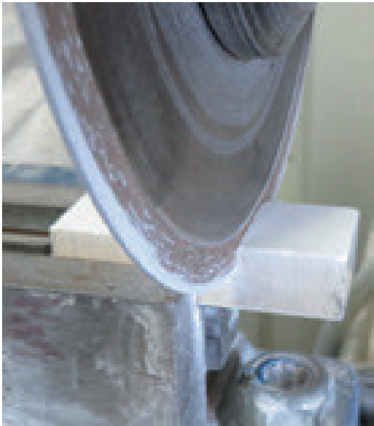
Green machining (cutting) of compacted GRANALOX® .
